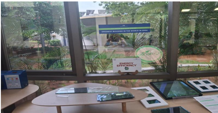
High-performance glass: Allows only visible light, not heat. This reduces heat load, lowers air-conditioning requirements, and enhances visual comfort by reducing glare.
